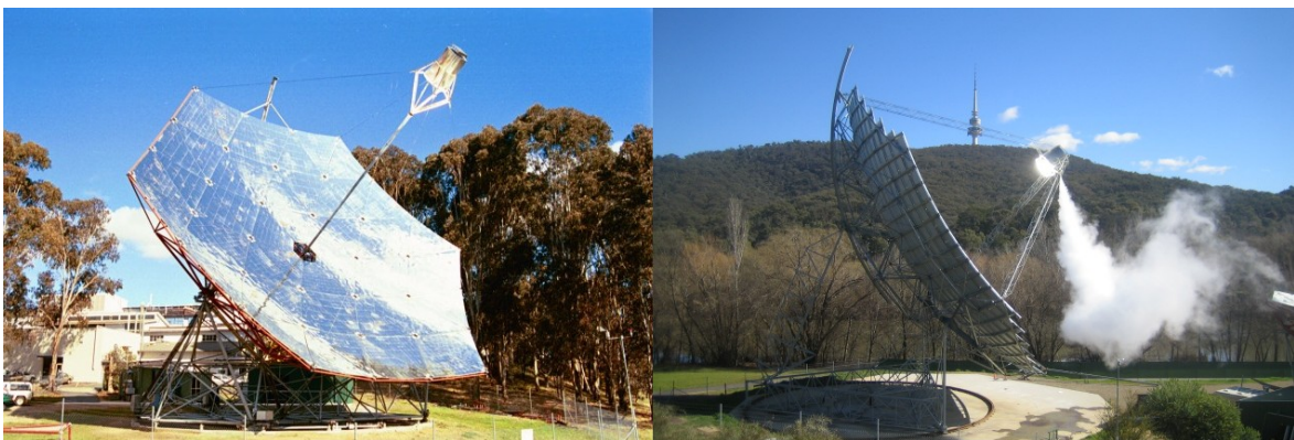
Figure 1: The 400m 2 "SG3" system (left) and the new 500m 2 "SG4" system (right) during experimental runs
