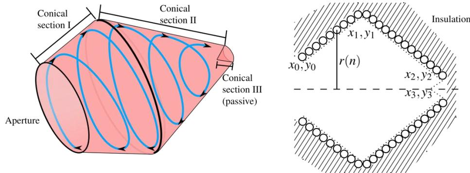
**Figure 1 (Left) Basic receiver geometry composed of three conical sections. (Right) Cavity receiver cross section, showing absorber tube loops.**
