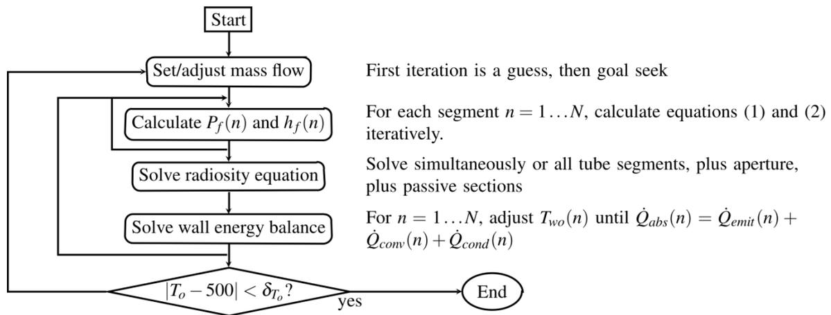
Figure 4 Solution procedure for the hydrodynamic model of the receiver tube
