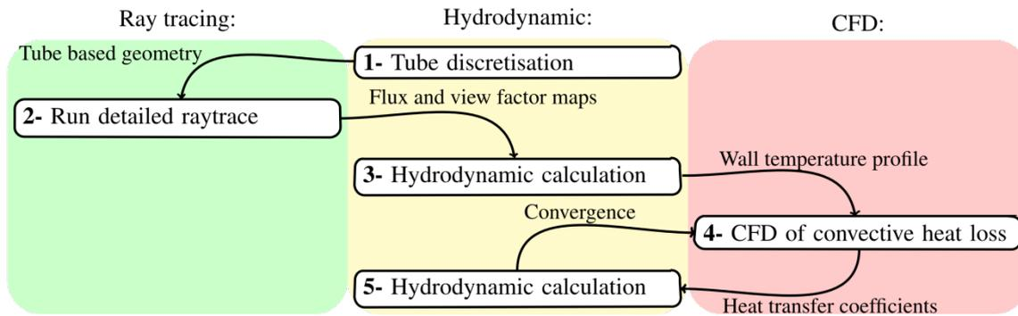
**Figure 2 Integrated model calculation stages across three simulation domains**
