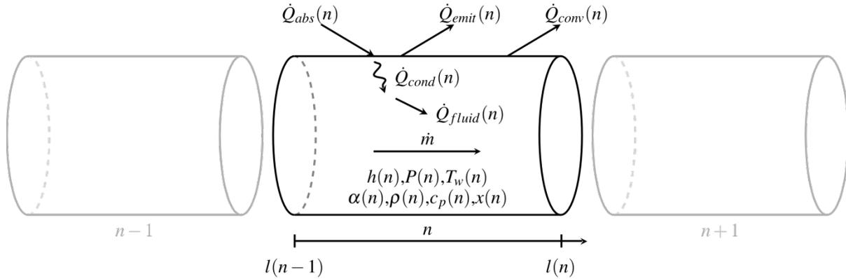
**Figure 3 Energy balance diagram for a tube segment  $n$  in the receiver geometry**
