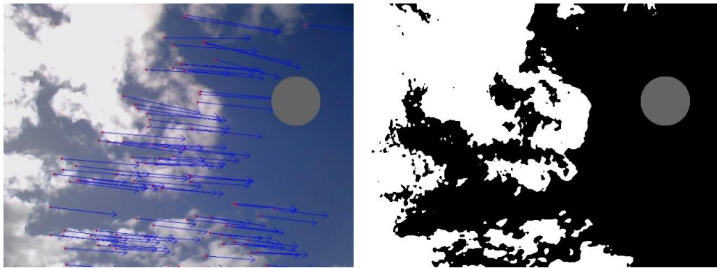
Figure 5. Image with velocity vectors and user defined region (left); detection image with user-defined region (right);
