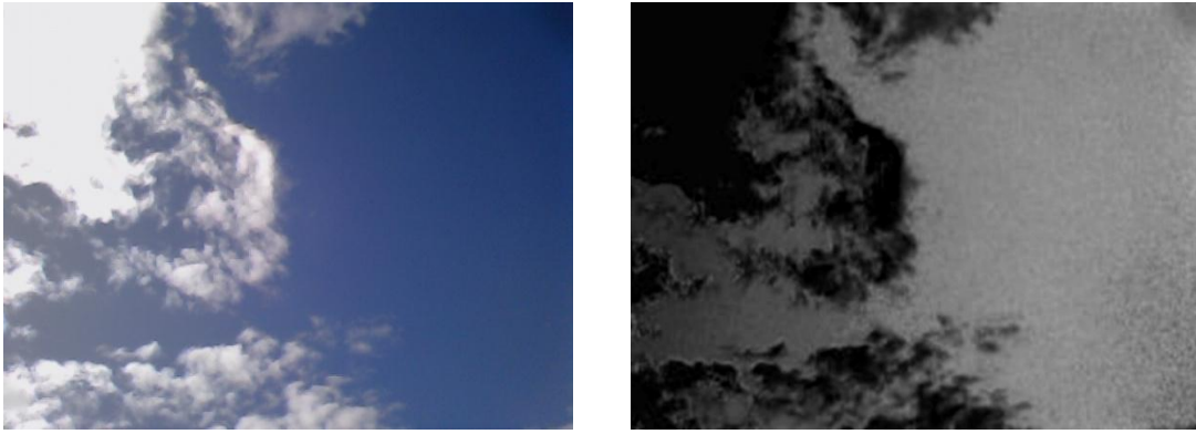
Figure 2. Original image (Left); B-R difference image scaled to 255 (right)
