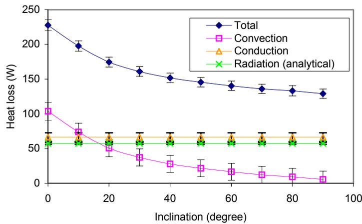
Fig. 5 Experimental heat loss for a cavity temperature of 450°C.
