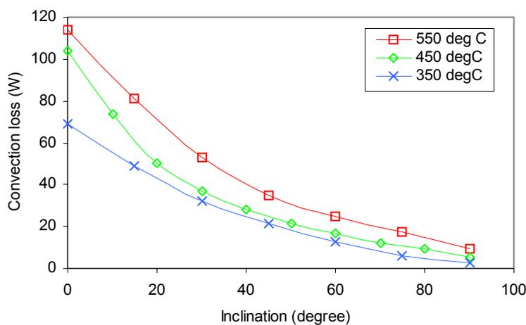
Fig. 6 Convection loss at various cavity temperatures
