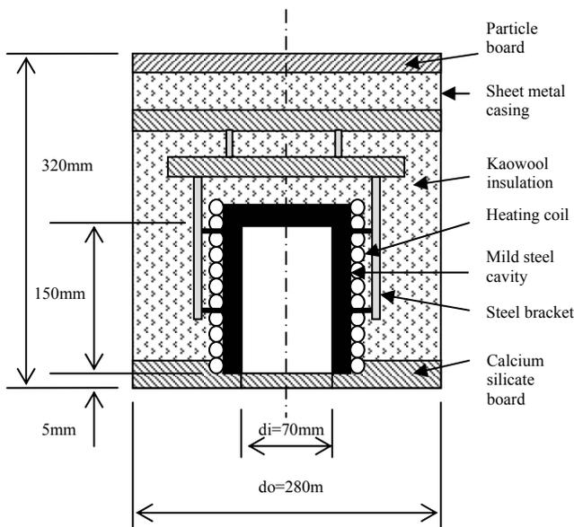
Fig. 1 Cross section sketch of model receiver.
