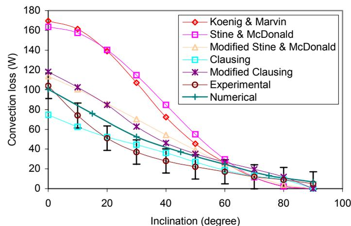
Fig. 6 Comparison of experimental convection loss at a cavity temperature of 450°C with other correlations.
