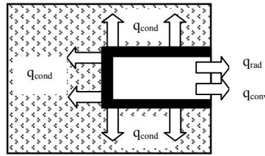
Fig. 3: Energy balance of model receiver.
