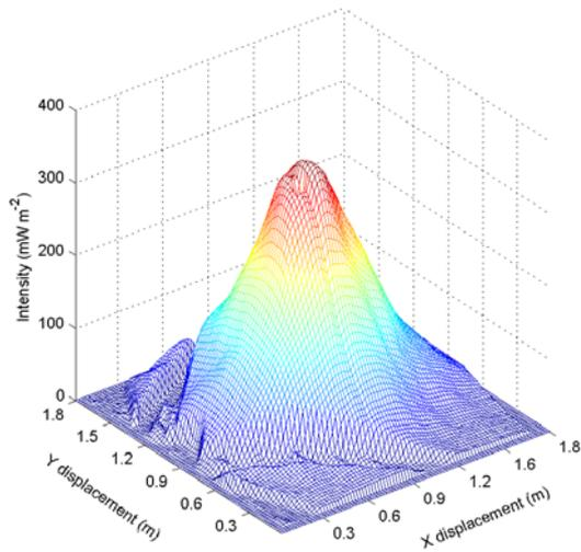
Figure 3: Surface plot of the flux distribution measured at the target of the ANU 400m<sup>2</sup> dish.
