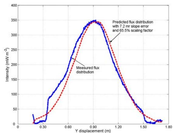
Figure 7b: Superposition of measured and predicted flux distribution along the Y-axis on the target.
