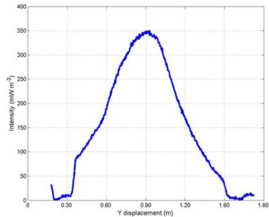
Figure 5b: Flux cross section at the image centroid point along the target Y-axis.
