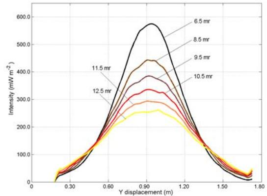
Figure 6b: Flux cross section along the Y-axis on the target.
