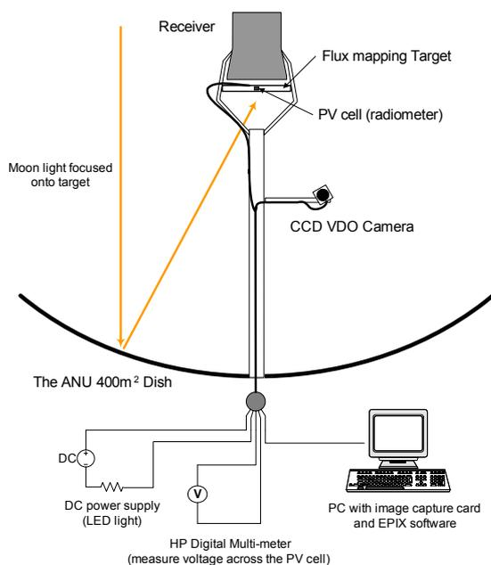
**Figure 2: Arrangement of the flux mapping equipment on the ANU 400 m<sup>2</sup> dish collector.**
