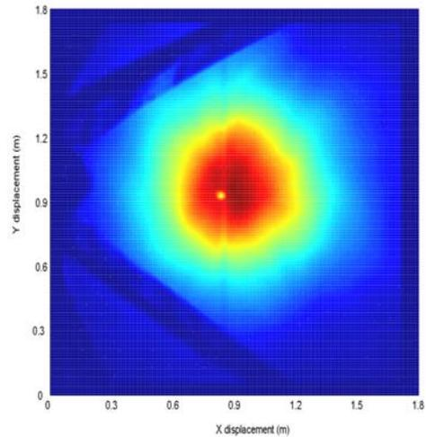
Figure 4: Contour plot of the flux distribution measured at the target of the ANU 400 m<sup>2</sup> dish.
