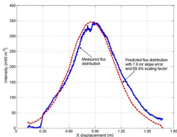
Figure 7a: Superposition of measured and predicted flux distribution along the X-axis on the target.
