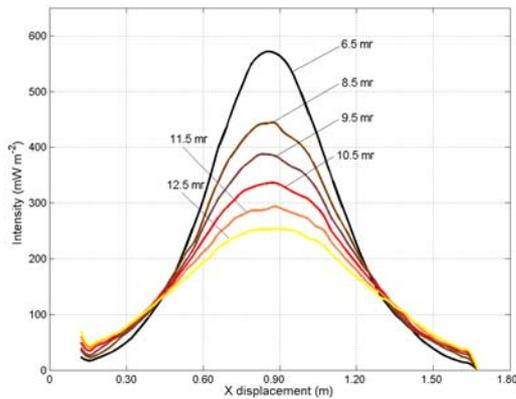
Figure 6a: Flux cross section along the Y-axis on the target.
