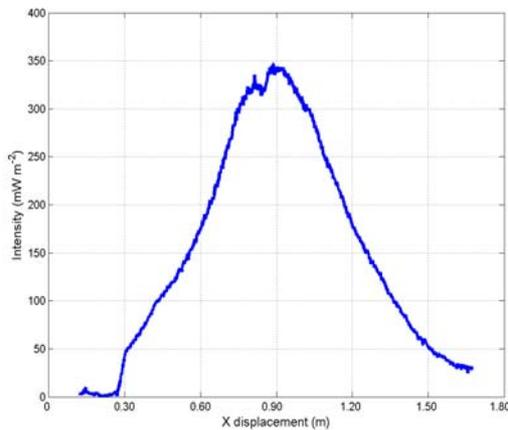
Figure 5a: Flux cross section at the image centroid point along the target X-axis
