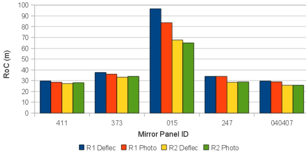
**Fig. 8. RoC results for 5 mirror panels compared to photogrammetry result.**
