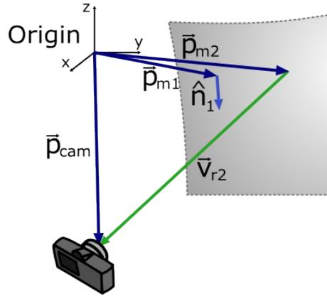
**Fig. 6. Extrapolation of surface out from know location.**
