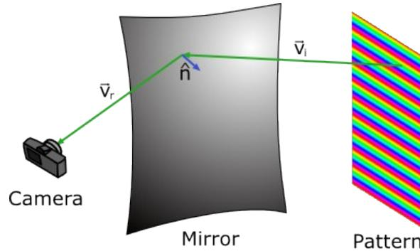
Fig. 2. Overview of measurement procedure.
