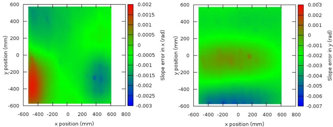
**Fig. 10. Mirror panel slope errors for panel 035 in two orthogonal directions.**
