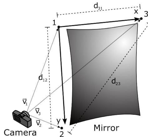
**Fig. 3. Camera locating dots positioned about mirror.**
