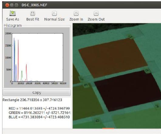
**Figure 6. The average pixel value in each of the three colour channels was sampled for each coloured region from a set of raw-format (.NEF) image files from the Nikon camera.**
