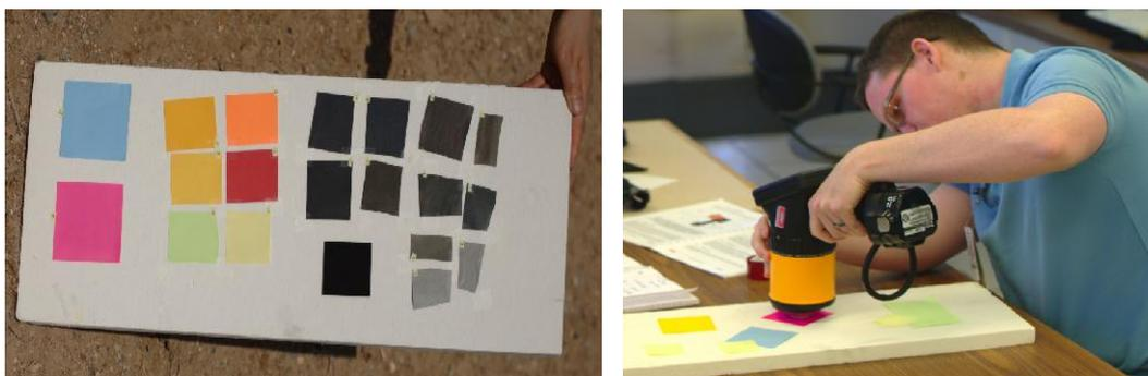
**Figure 3. (a) Grey and coloured samples used to evaluate the coupon method. The very dark square is the Pyromark 2500 painted sample. (b) Measurement of the samples using the SOC 410-Solar handheld 7-band solar reflectometer.**
