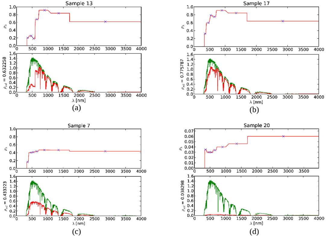
**Figure 4. Reflectivity spectra from 410-Solar measurements for (a) orange paper sample (b) green paper sample (c) grey paper sample (d) Pyromark 2500 sample. The lower part of each plot shows the AM1.5 ASTM G173 air mass 1.5 solar spectrum together with the calculated reflected spectrum; at the lower left of each plot is the calculated solar-weighted reflectivity.**
