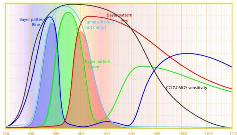
**Figure 8. Typical CCD response curve (relative spectral response versus wavelength in nm). The pale blue 'hot mirror' line shows the visible-range light filter which suppresses the response of the CCD to longer-wavelength irradiation (Source:ir-photo.net)**
