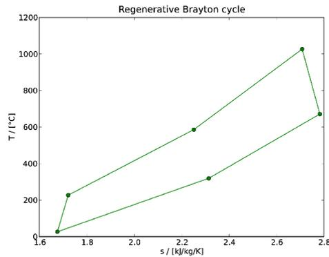
**Figure 3. Regenerative air Brayton cycle with regenerator effectiveness of 80%. The cycle efficiency is 40.88 %. For plotting, curved lines have been approxiated as straight.**
