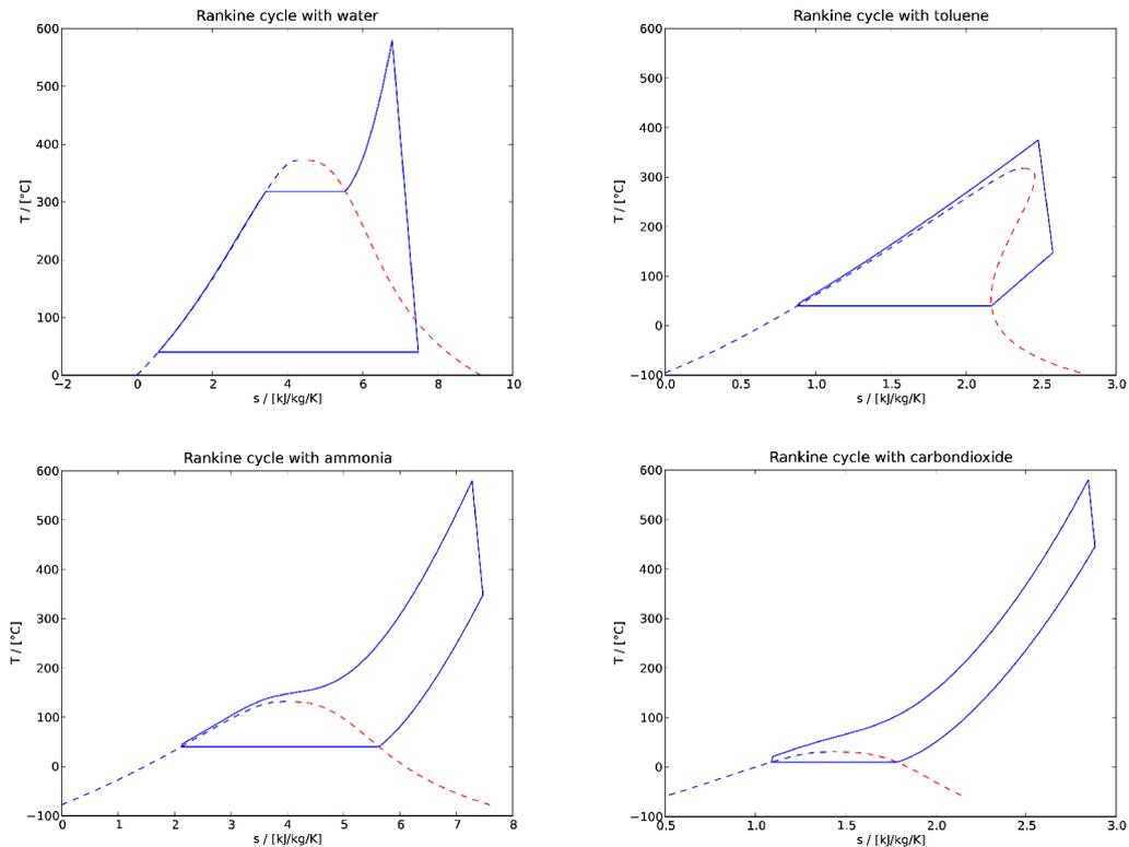
**Figure 1. Simple Rankine cycles for water, toluene, ammonia, and carbon dioxide. The cycle temperature limits are  $580 \text{ }^\circ\text{C}$  and  $40 \text{ }^\circ\text{C}$ ; the upper pressure limit is 150 bar, and the vapour mass fraction at the turbine outlet is not allowed below 90%.**
