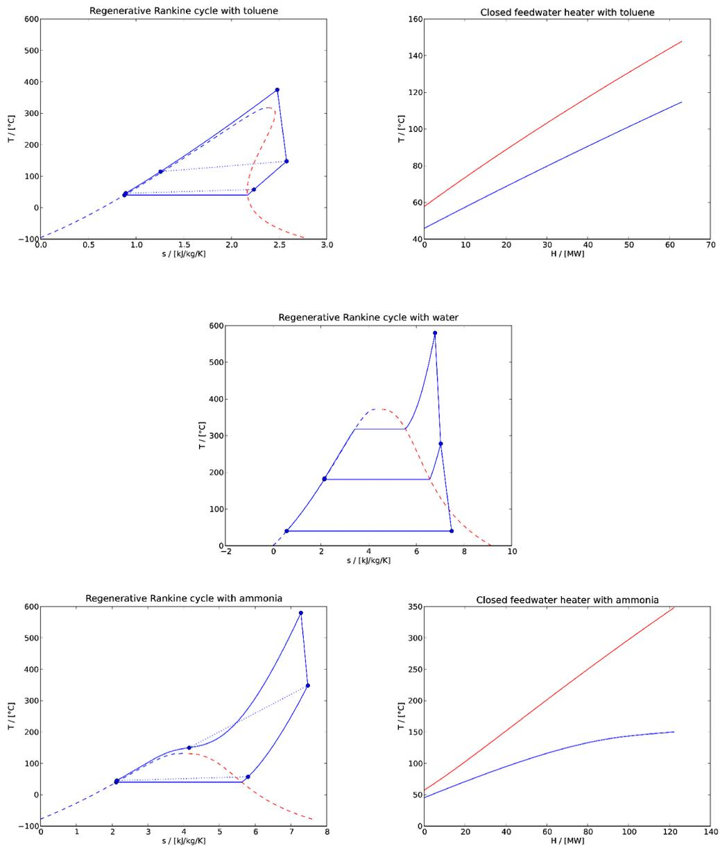
**Figure 2. Regenerative Rankine cycle models with the same cycle limits as earlier. The feedwater heater gives a greater improvement for the non-water cycles. Heat exchanger profiles are shown for the toluene and ammonia cycles. In the water cycle, an open feedwater heater is assumed.**
