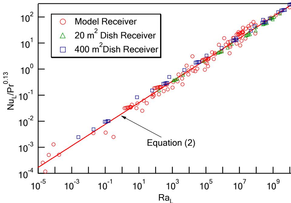
**Figure 6 Comparison between the prediction by Equation (2) and the numerical results.**
