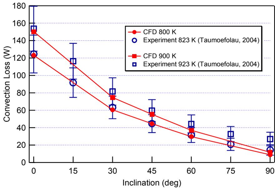
**Figure 3 Comparison for the case of the model receiver with varying cavity wall temperature.**
