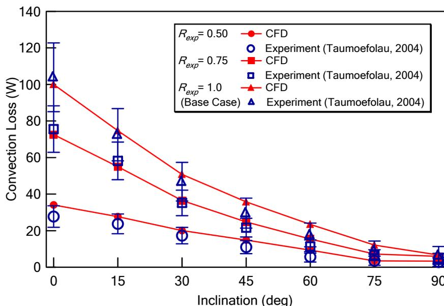
Figure 2 Comparison for the case of the model receiver with varying aperture areas.
