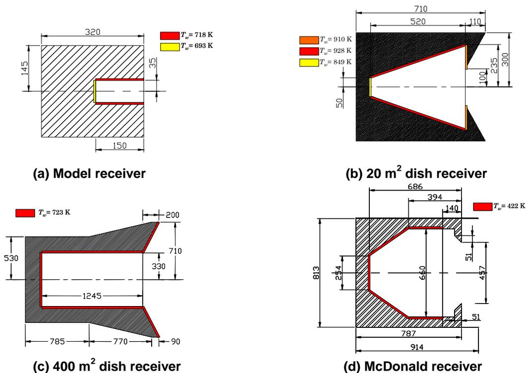
Figure 1 Configurations of receivers used in the study.
