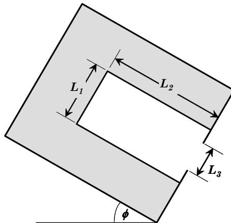
Figure 5 Denotation of cavity geometrical parameters used in the definition of the ensemble cavity length scale  $L_s$ .
