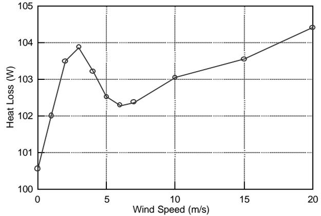
**Figure 6 The Relationship between Wind Speed and Heat Loss for Model Receiver with Wind Normal to the Aperture Plane.**
