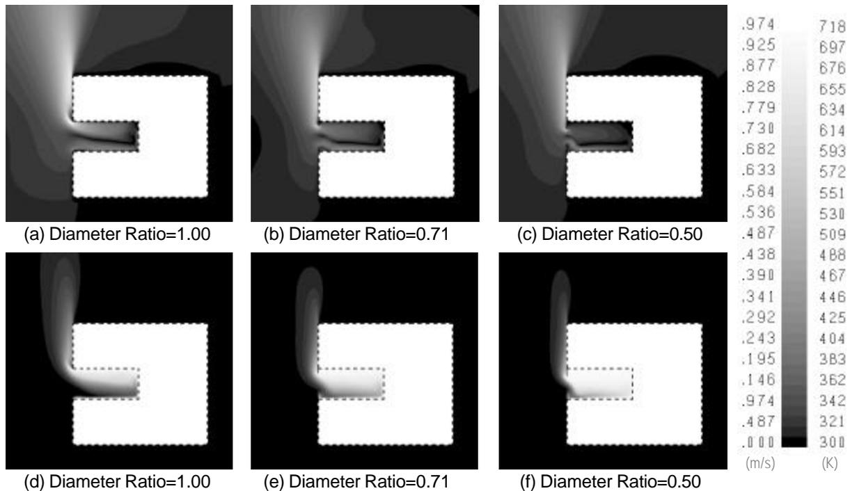
**Figure 3 Contour Plot of Velocity Magnitude ((a)-(c)) and Temperature ((d)-(f)) at Symmetrical Plane for Model Receiver with Different Aperture to Cavity Diameters Ratio.**
