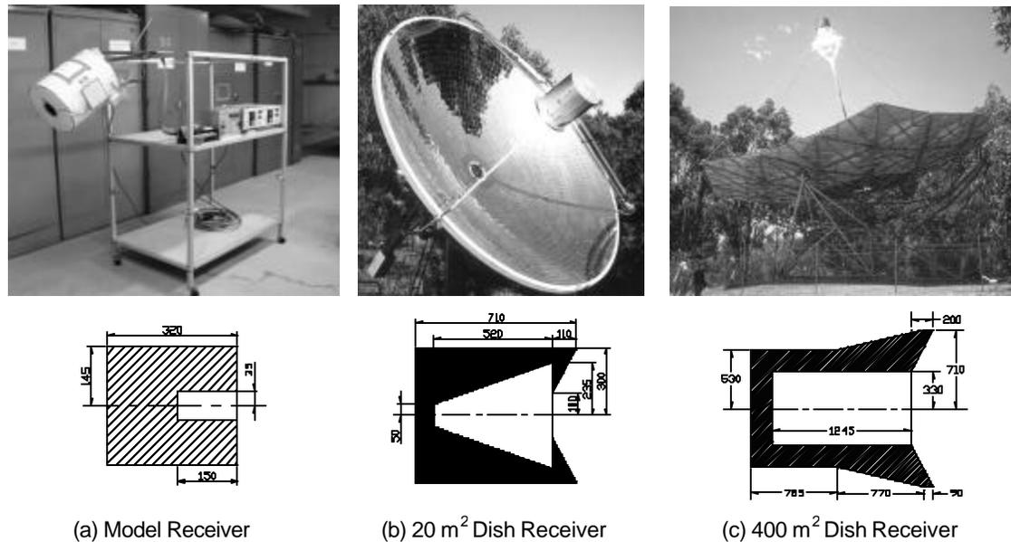
**Figure 1 Three Receiver Systems and Cross Sectional Diagram of All Three Receiver Models.**
