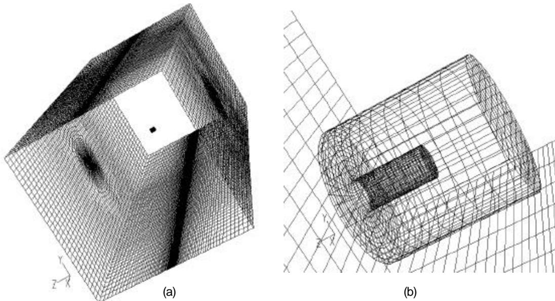
**Figure 2 Typical computational grid for combined convection study of model receiver:
