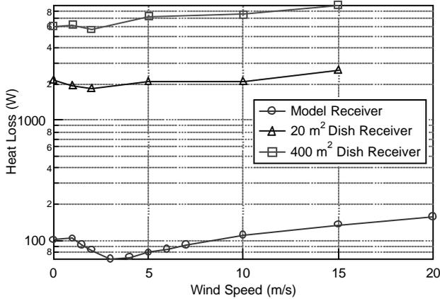
**Figure 5 The Relationship between Wind Speed and Heat Loss for All Three Receivers with Wind Parallel to the Aperture Plane.**
