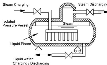
Fig. 1: Scheme of variable-pressure accumulator (Steinmann & Eck 2006)
