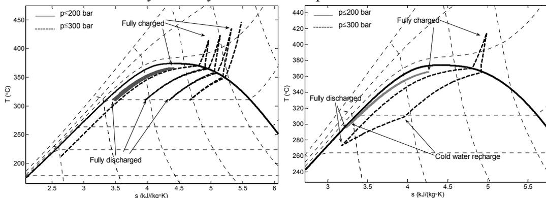
Fig. 2: T-s diagram of the accumulator charging/discharging process for super-critical and sub-critical pressure limited storage vessels (a) without (b) with cold water recharge for super-critical and sub-critical pressure limited storage vessels.
