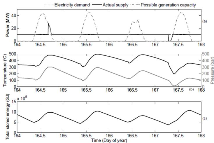
Fig. 4: Four-day simulation of winter period (13-16 June 1997) in Alice Springs. (a) power generated for a constant electricity demand, (b) storage temperature and pressure and (c) total stored energy.
