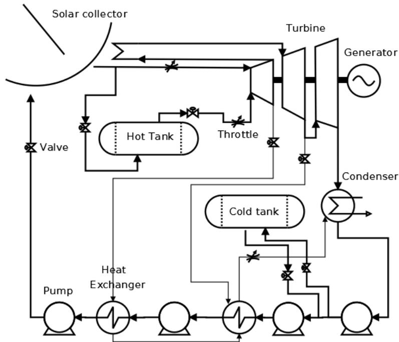
Fig. 3: System layout for dynamic model of a two-tank storage system utilising compressed liquid.
