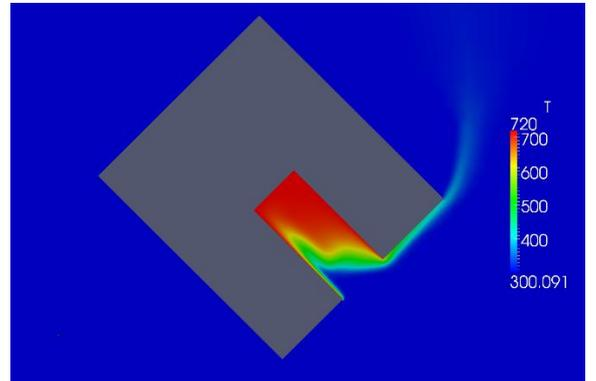
Figure 6. 45° Inclined Cavity without an Air Curtain
