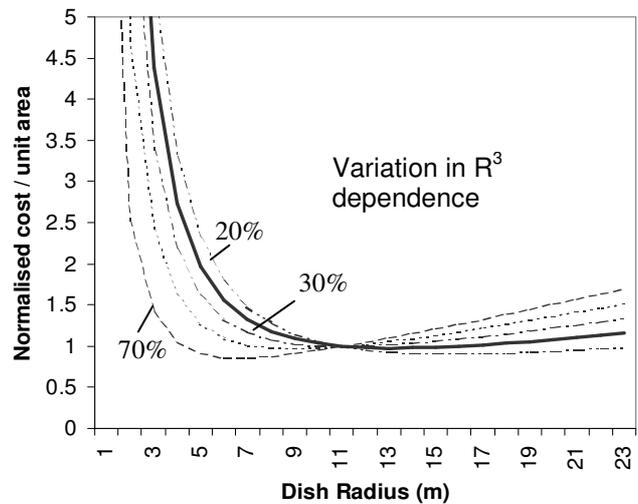
Figure 2. Normalised per unit dish area cost as a function of dish radius, for a range of fractional dependencies on R<sup>3</sup>. Fixed costs and R<sup>1</sup> dependant fractions are kept in the ratio 2:1. and R<sup>2</sup> costs kept at 20%.
