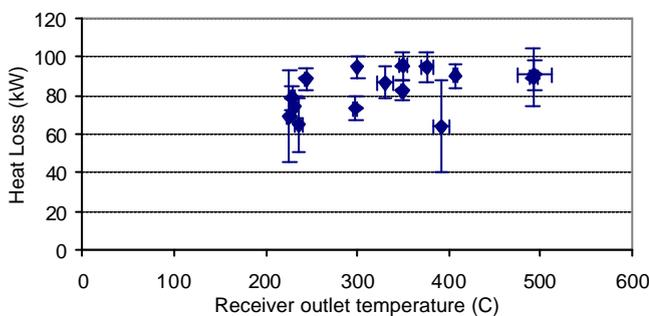
Figure 3. Recent measurements of combined optical and thermal losses for the ANU 400m<sup>2</sup> dish system.
