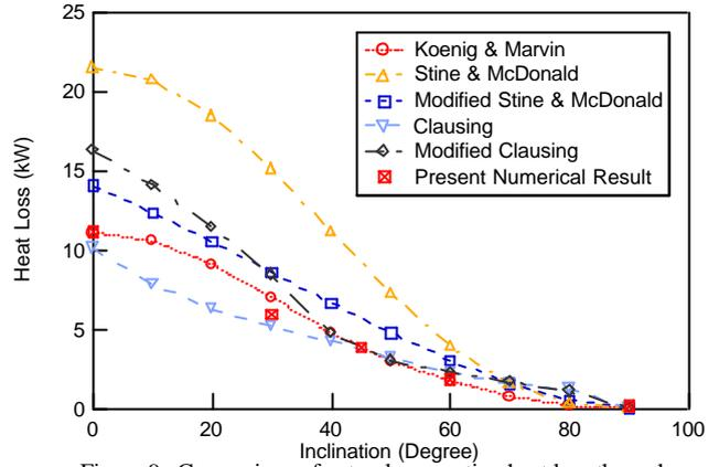
Figure 9. Comparison of natural convection heat loss through the aperture for 400 m<sup>2</sup> dish receiver.
