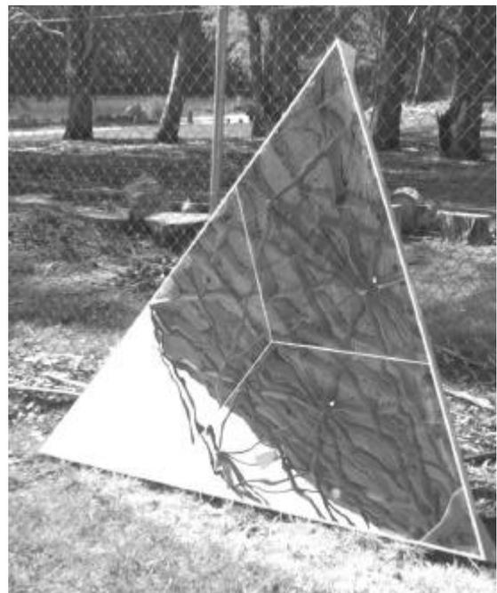
Figure 2: Triangular prototype GOML solar reflector element for ANU's 400 m<sup>2</sup> dish.
