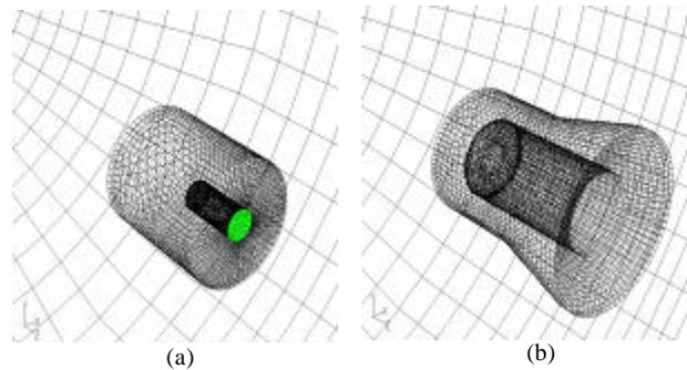
Figure 6. Typical computational grids for (a) model receiver and (b)  $400 \text{ m}^2$  dish receiver.
