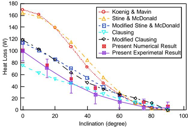
Figure 8. Comparison of natural convection heat loss through the aperture for model receiver.
