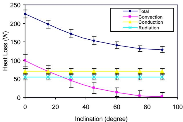
Figure 5. Experimental heat loss for a cavity temperature of  $445^{\circ}\text{C}$ .
