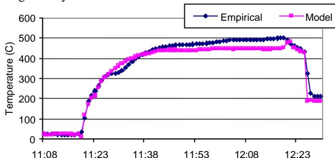
Figure 11. Comparison of experimental and modelled receiver exit temperature for 9 Jan 2003. Dish on the sun from 11.18–12.19 with approximately constant 1000Wm<sup>-2</sup> insolation.
