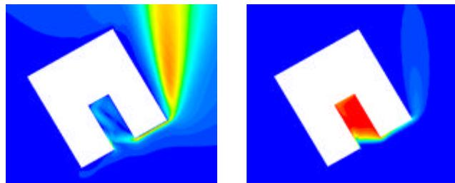
Figure 7. Contour plots at symmetric plane for model receiver at  $60^{\circ}$  inclination: (a)- velocity magnitude, (b) temperature.
