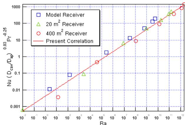
Figure 10. Comparison of prediction by the present correlation and numerical results of three receivers.
