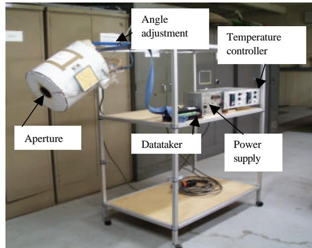
Fig. 4 Experimental setup for laboratory investigation of convection losses.
