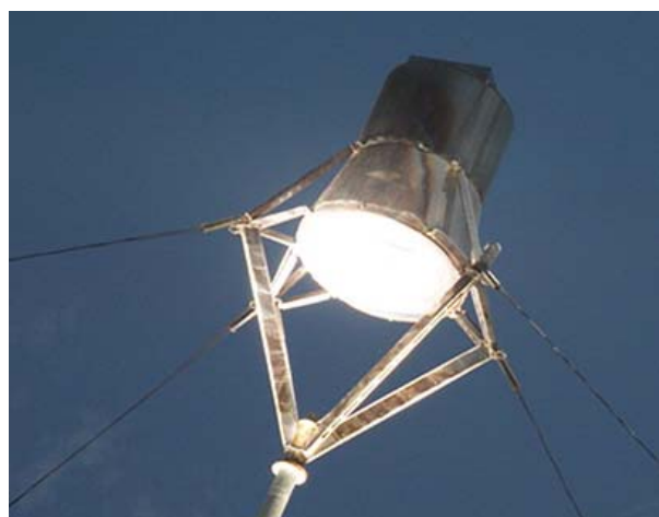
Figure 2. SG3 monotube boiler receiver during operation.
