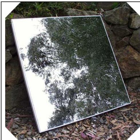
Figure 8. Square mirror panel (1.1x1.1 m.) used for flux measurement studies.
