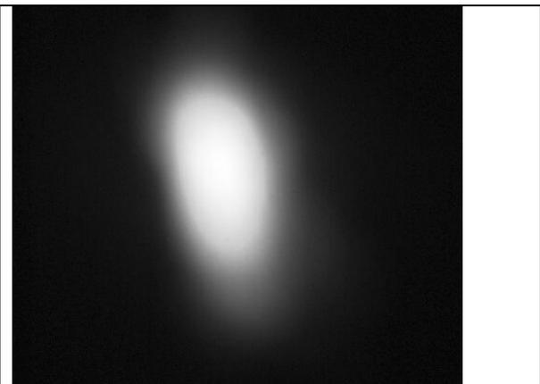
Figure 9. Flux distribution for the square mirror panel shown in Figure 8. Panel-target distance = 13.8 m. Target dimensions = 900x900 mm.
