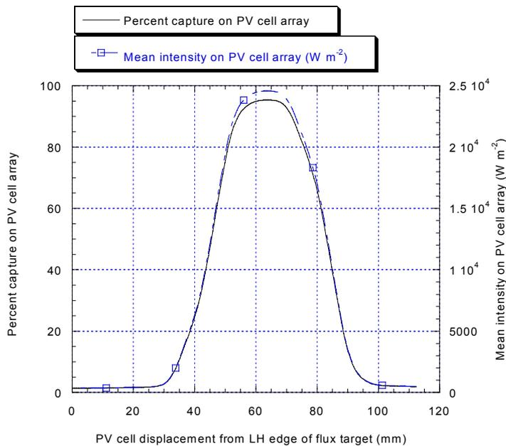
**Figure 7. Both mean cell array intensity, and percentage radiation capture on a 38 mm wide x 1600 mm long PV cell array scanned across the flux line shown in Figure 5.**
