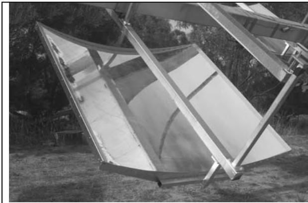
**Figure 1. Glass-On-Metal-Laminate (GOML) trough concentrator for concentrating photovoltaic power generation.**
