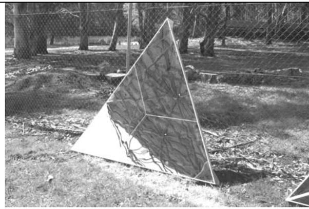
**Figure 2. Foam-cored mirror panel developed for large area solar dish applications.**
