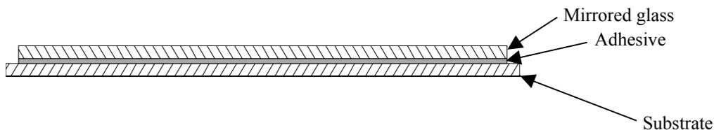
**Figure 3. Basic construction of a glass-on-metal-laminate (GOML) structure.**
