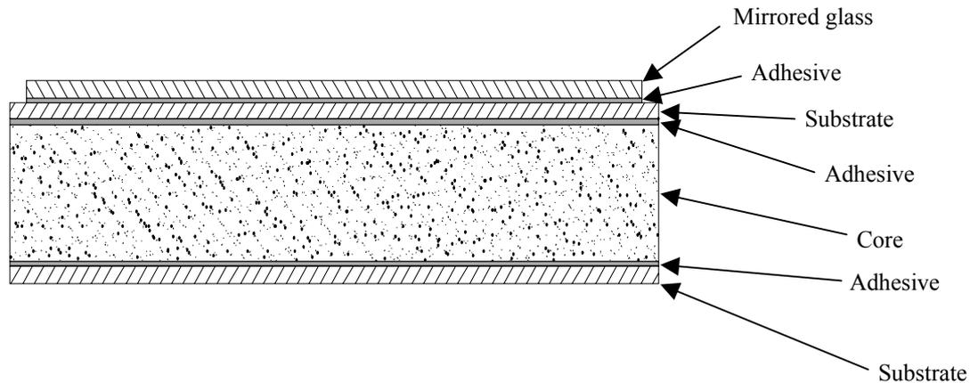
**Figure 4. Basic construction of a foam-cored composite sandwich structure used for fabricating 3-dimensionally curved, self-shape-holding mirror panels or facets.**
