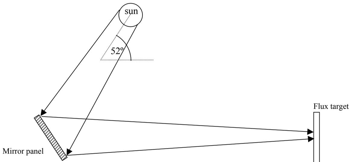
**Figure 12. Arrangement of mirror panel and flux target for flux map measurement.**
