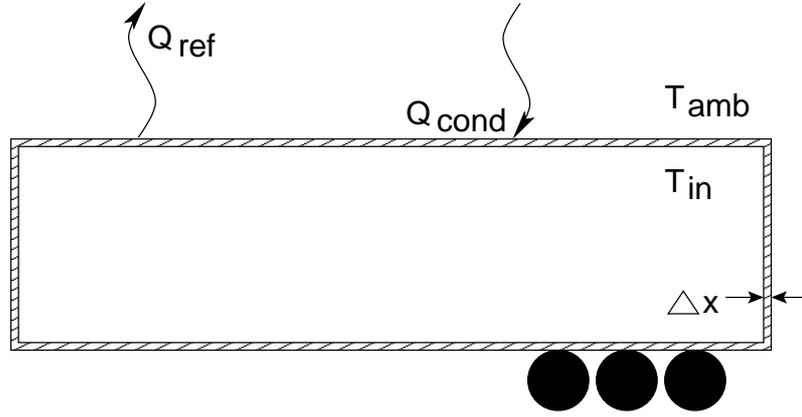
Figure 1: Basic thermodynamic model of the trailer.
