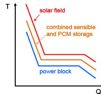
Fig. 7: Heat transfer in a three-part storage system
