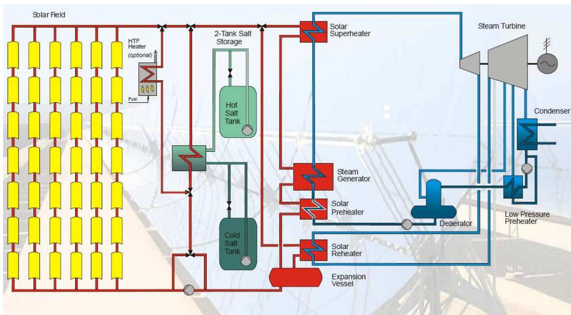
Fig. 2: A plant flow diagram for Andasol-1 and similar plants.
