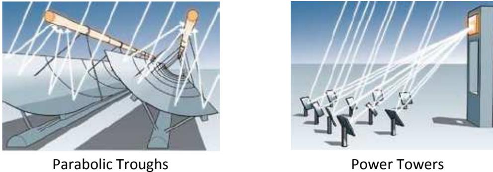
Fig. 3: Operating principles of parabolic troughs and power towers (Images: Siemens).
