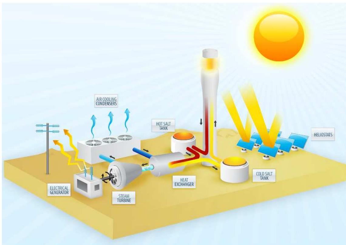
Fig. 4: The operating principle of a molten salt power tower (Image: Sharon Wong).
