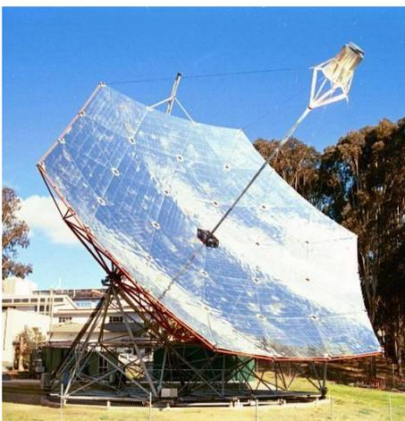
Successful ammonia dissociation experiments have been carried out using a 20m<sup>2</sup> paraboloidal dish concentrator (Lovegrove *et al.* 2004). ANU's ammonia technology has been licenced to Wizard Power Pty Ltd ([www.wizardpower.com.au](http://www.wizardpower.com.au)), who have secured support via the Australian Federal
