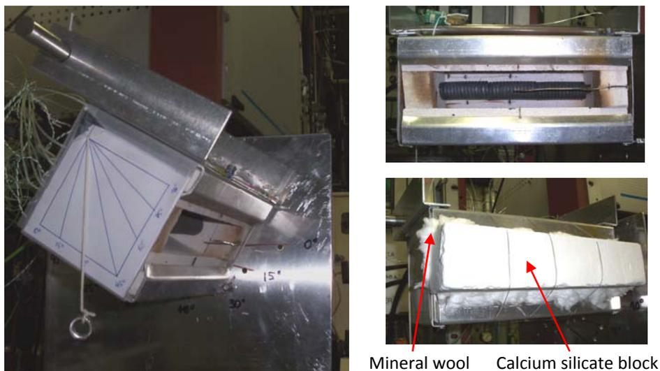
Figure 2—2. Left : The apparatus used to set the angle of inclination for the small-scale receiver, 30 degrees in the photo. Top right : A front view of the cavity and heating elements for the small-scale receiver. Bottom right : The blocked cavity set up used to measure conduction losses.
