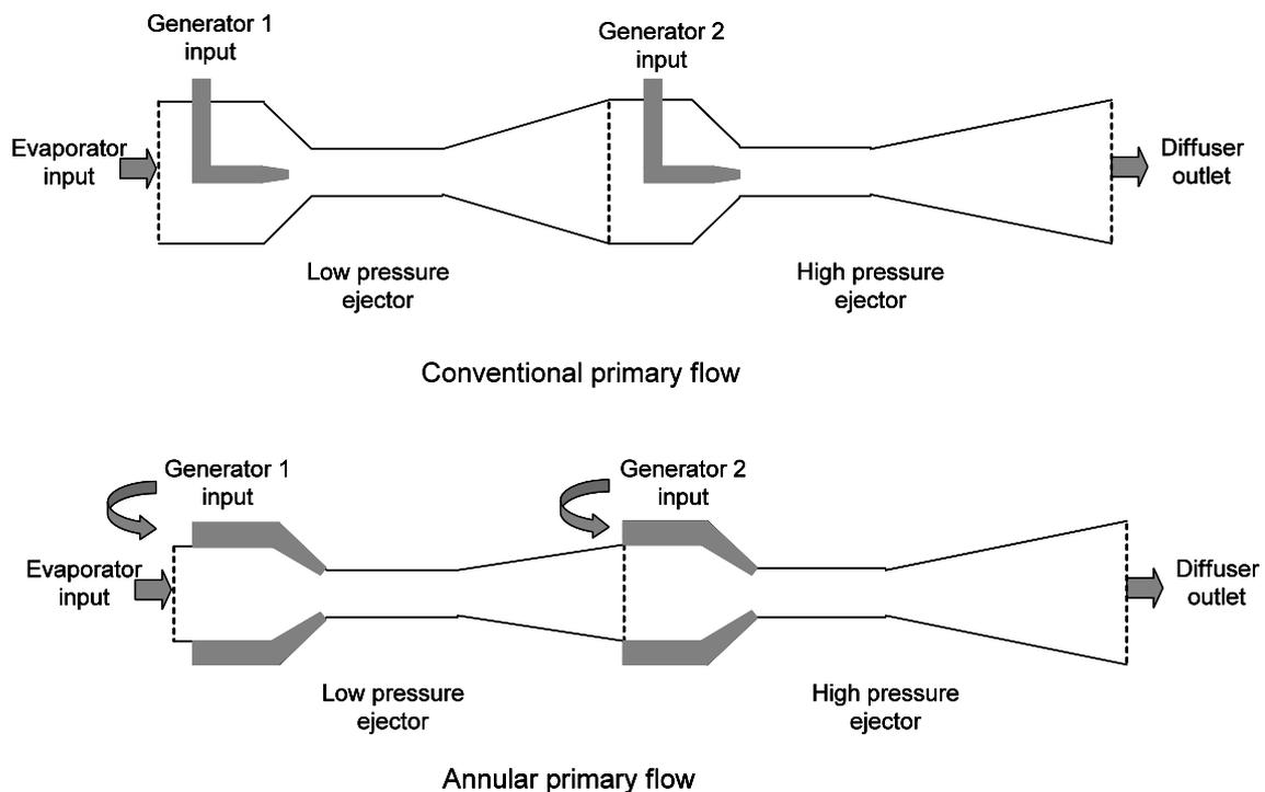
Figure 9. Coaxial designs for compound ejector
