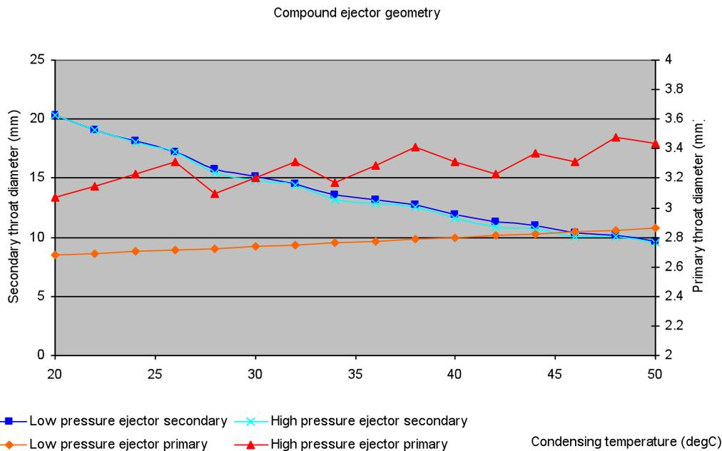
Figure 6. Design geometry for the compound family of ejectors, each optimised for a given condensing temperature.
