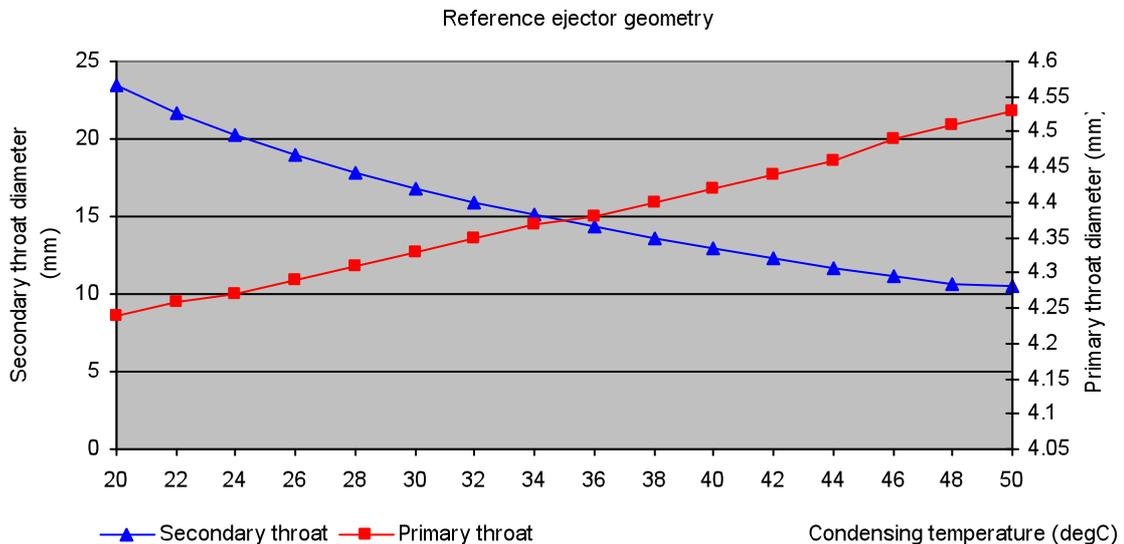
Figure 3. Design geometry for the reference family of ejectors, each optimised for a given condensing temperature
