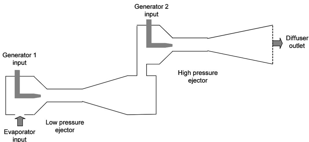
Figure 2. Schematic of a compound ejector
