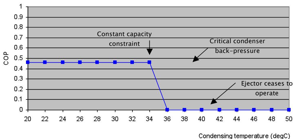
Fig.1. Typical operating characteristics of ejectors designed for fixed condensing temperatures
