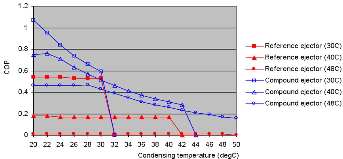
Figure 8. Comparison of operating performance of reference and compound ejectors designed for condensing temperatures 30°C, 40°C and 48°C.
