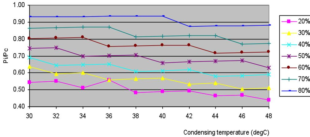
Figure 5. Determining the operational intermediate pressure  $P_i$  as a proportion of the condensing pressure  $P_c$  and condensing temperature.
