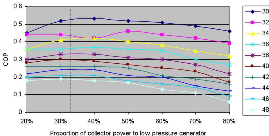
Figure 4. Proportioning of the collector power between the low and high pressure ejectors shows a broad optimum COP
