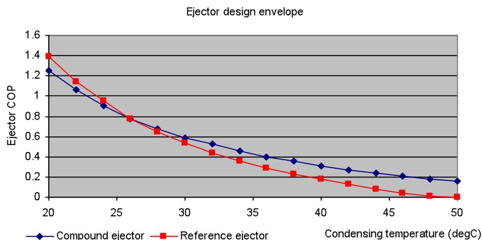
Figure 7. Performance limits are defined by a design envelope shown for the reference and compound ejectors at condensing temperatures.
