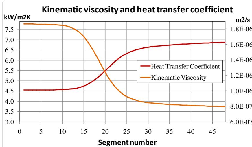
**Fig. 4. Molten salt kinematic viscosity and heat transfer coefficient.**
