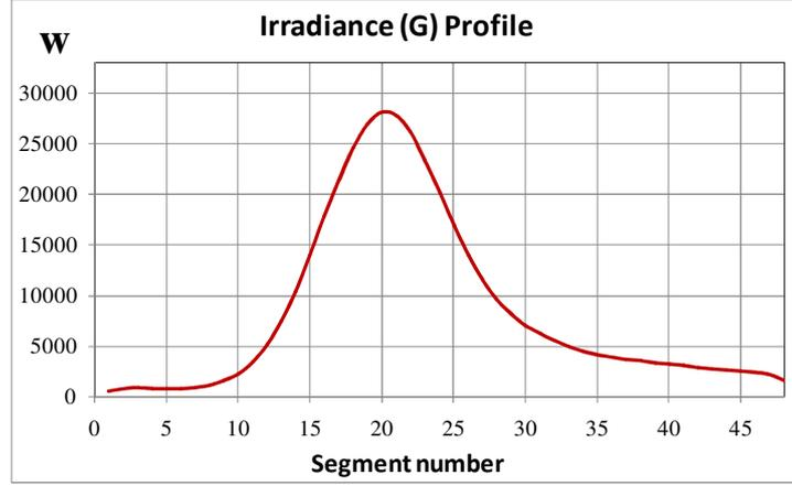
**Fig. 2. Irradiance for each tube segment, numbered vertically upwards from receiver opening.**
