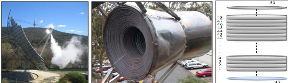
**Fig.1. The ANU SG4 dish (left), its current receiver (center) and the model geometry (right).**
