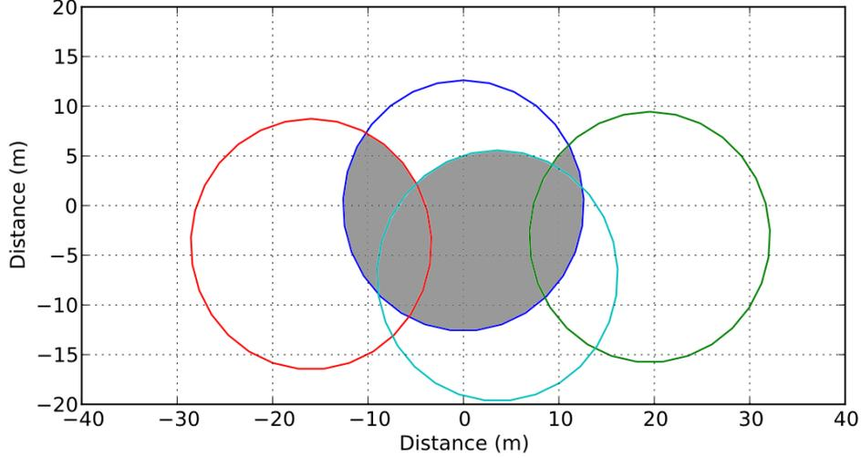
**Figure 3. Graphical representation of polygon overlap in the sun-view coordinate system for a discrete time sample. Overall shading is the area of the union of shade polygons that are determined by calculating the intersection of each polygon with the central polygon.**
