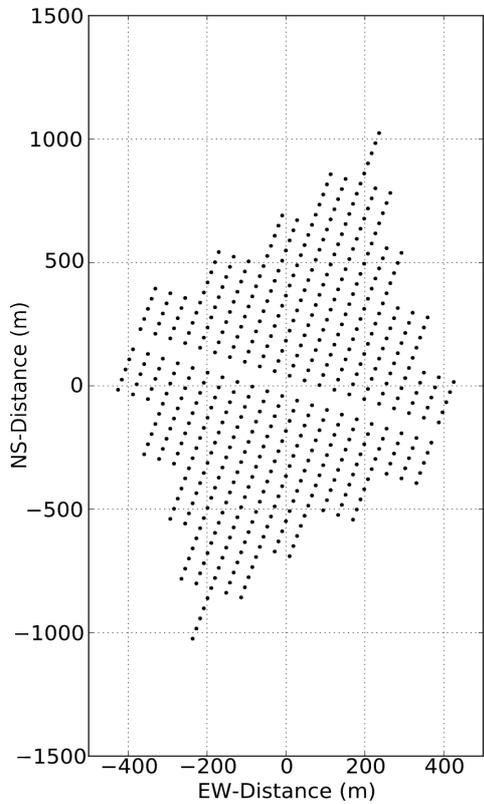
**Figure 4. The calculated optimum first-order lattice for the simulated energy transport network and power plant site (top) and the arrangement of the dishes comprising the power plant (bottom).**
