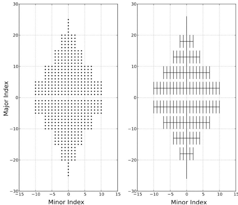
**Figure 1. Dish-field array. Each dot represents a paraboloidal dish (left) and lines represent the underlying energy transport network (right). Pipe links enter the power block at (0,1) and (0,-1) for the top and bottom half, respectively.**
