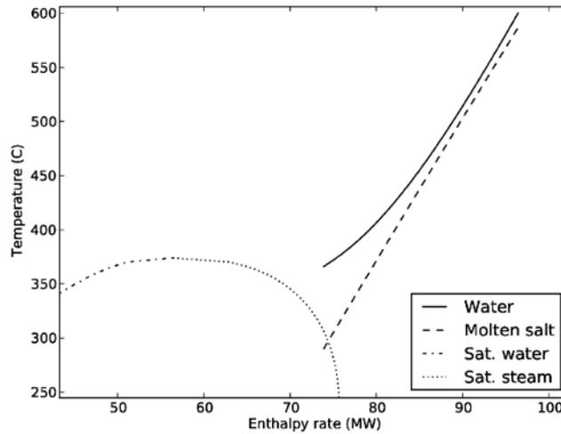
**Fig. 1. Temperature-enthalpy diagram showing heat transfer to molten salt from superheated steam.**
