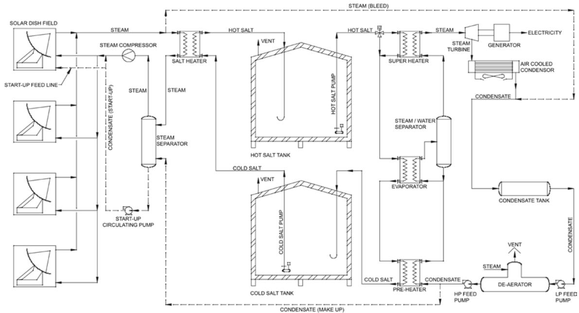
**Fig. 3. Process Flow Diagram for the Whyalla Energy Storage project**
