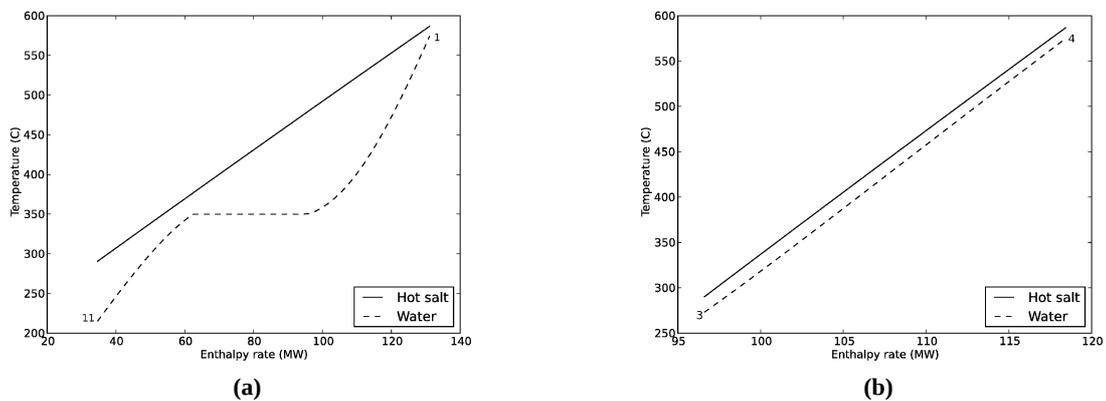
Figure 7. Heat transfer temperature-enthalpy curves for the two boiler stages in the subcritical cycle: (a) main boiler and (b) reheater.
