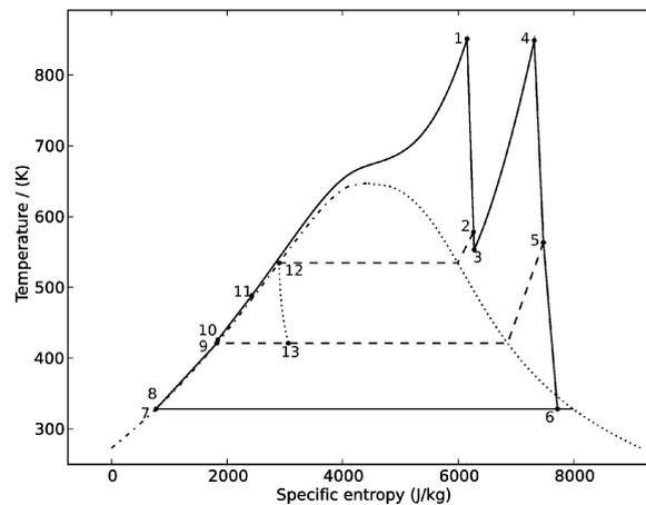
Figure 8. Temperature-entropy diagram for a reheat-regenerative supercritical Rankine cycle.
