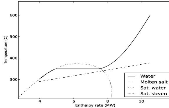
**Figure 1. Temperature-enthalpy diagram showing how the 'pinch point' limits the upper temperature of the energy storage medium. Shown is the cooling curve of 165 bar steam.**
