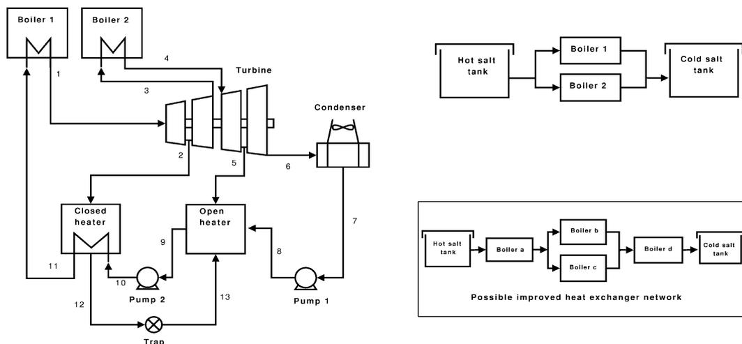
**Figure 5. Schematic diagram of thermal power cycle (left), a simple heat exchanger network (top right). Bottom right shows a generic heat exchanger network for improved heat transfer.**
