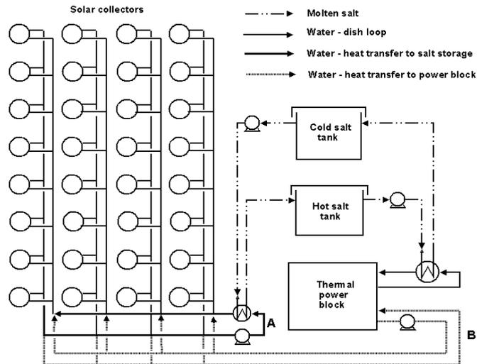
**Figure 2. Basic process flow sheet showing interconnectivity of a solar field, molten salt storage system and thermal power block.**
