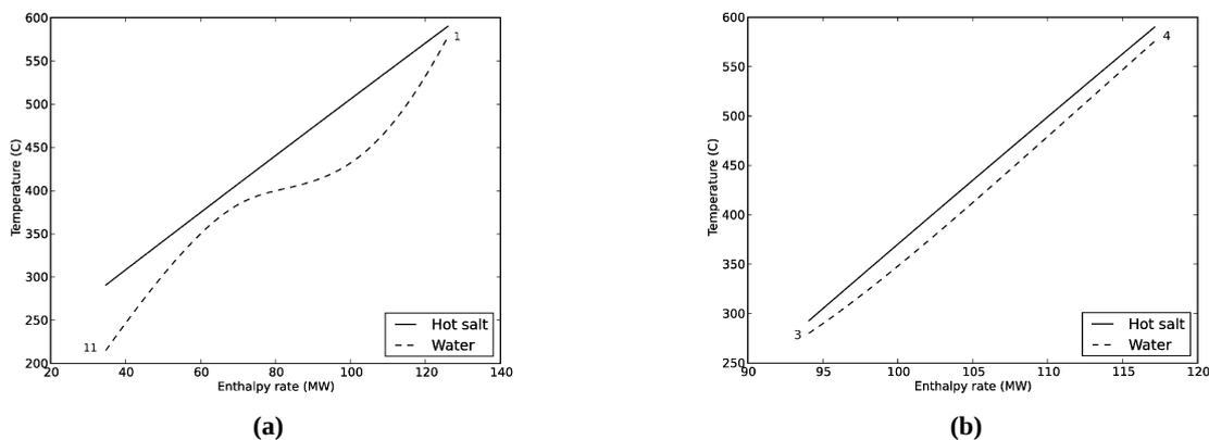
Figure 9. Heat transfer temperature-enthalpy curves for the two boiler stages in the supercritical cycle, (a) main boiler, and (b) reheater.
