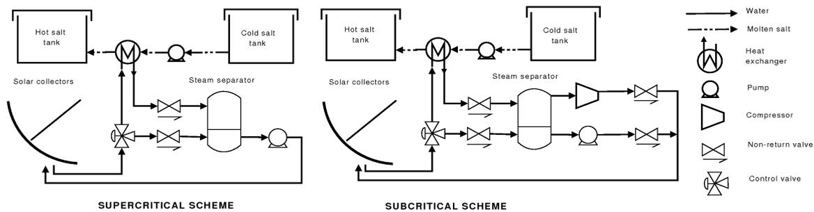
**Figure 4. Details of process flow for steam charging of molten salt storage**
