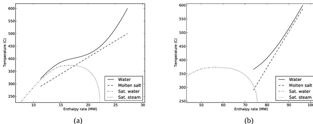
**Figure 3. Temperature-enthalpy diagrams showing heat transfer to molten salt from (a) supercritical steam at 300 bar, and (b) superheated subcritical steam at 165 bar.**
