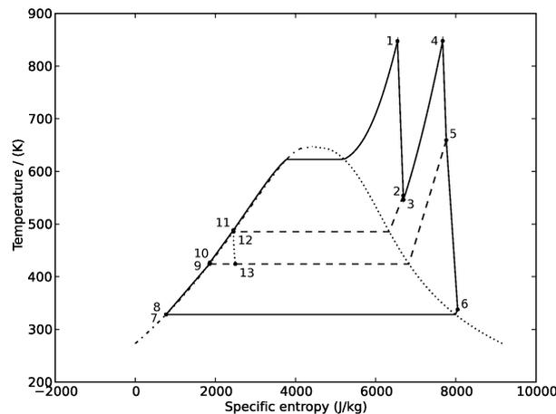
Figure 6. Temperature-entropy diagram for a reheat-regenerative subcritical Rankine cycle
