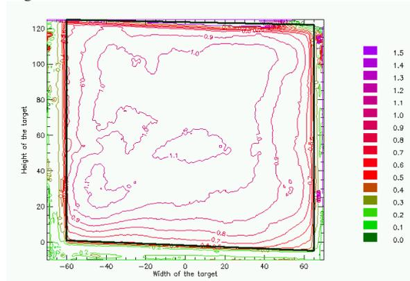
**Figure 4:** Measured radiation flux intensity at the focus without the secondary reflector. Units are normalised against the median.
