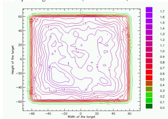
**Figure 9:** Simulated flux intensity with the secondary reflector. Units are normalised to the median of the receiver area shown in figure 8.
