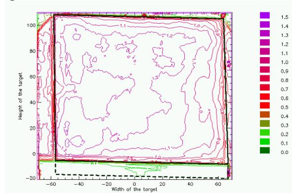
**Figure 5:** Measured radiation flux intensity at the focus with the secondary reflector. Units are normalised again using the median of the data in figure 4.
