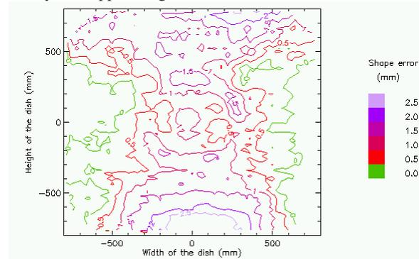
**Figure 7:** Shape error of the dish after mirrors were applied.
