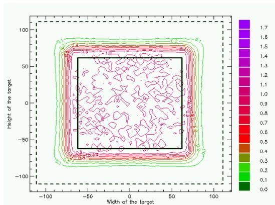
**Figure 2:** Flux intensity predicted by ray tracing if the mirror had the ideal shape. Units are normalised against the median.
