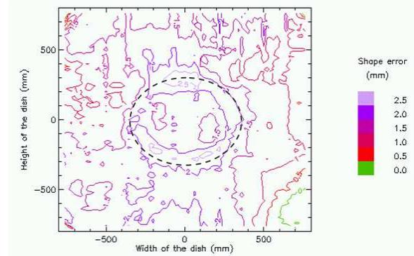
**Figure 6:** Shape error of the dish before mirrors were applied. The dashed line indicates the clear impression left by the support ring mounted on the back of the dish.
