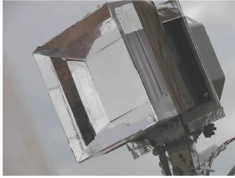
**Figure 3:** Secondary reflector mounted on the Lambertian target.
