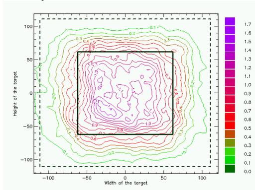
**Figure 8:** Simulated flux intensity without the secondary reflector. Units are normalised to the median of the area corresponding to receiver (shown in bold).
