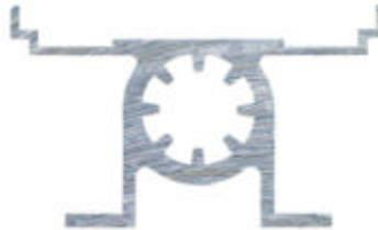
**Figure 3. Cross-section of the ANU receiver.**
