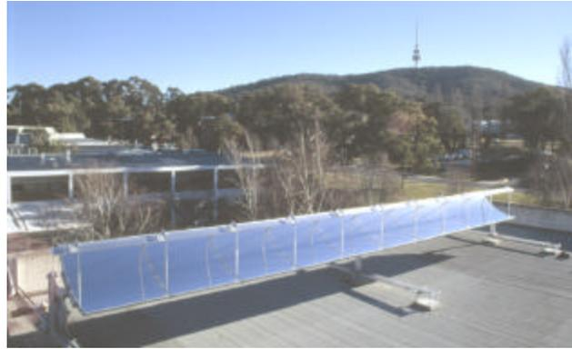
**Figure 1. Prototype CHAPS collector at ANU.**
