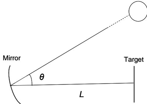
**Fig. 3: Configuration for mirror panel flux mapping**
