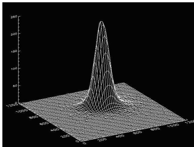
**Fig. 5: Surface plot (unscaled) of the lunar flux distribution of SG4 dish, measured 4 September 2009. At the time of image capture the moon was 97.6% full and had an angular radius of 4.35 mrad.**
