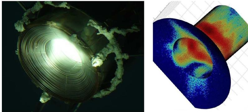
**Fig. 7: (Left) Camera image of the SG4 dish steam receiver on sun. (Right) contour plot of flux distribution on the receiver surface generated by Tonatiuh ray tracing.**
