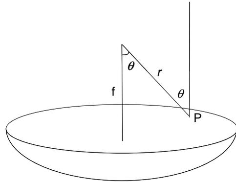
**Fig. 4: Equivalent situation on dish paraboloid**
