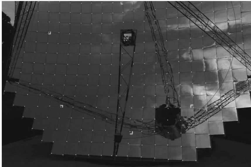
**Fig. 2: Camera image with flash of SG4 dish with retro reflective targets located at panel corners.**
