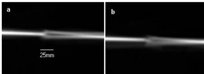
**Figure 7 Flux images for 25mm gap,  $0^\circ$  (a) and  $10^\circ$  (b) orientations.**
