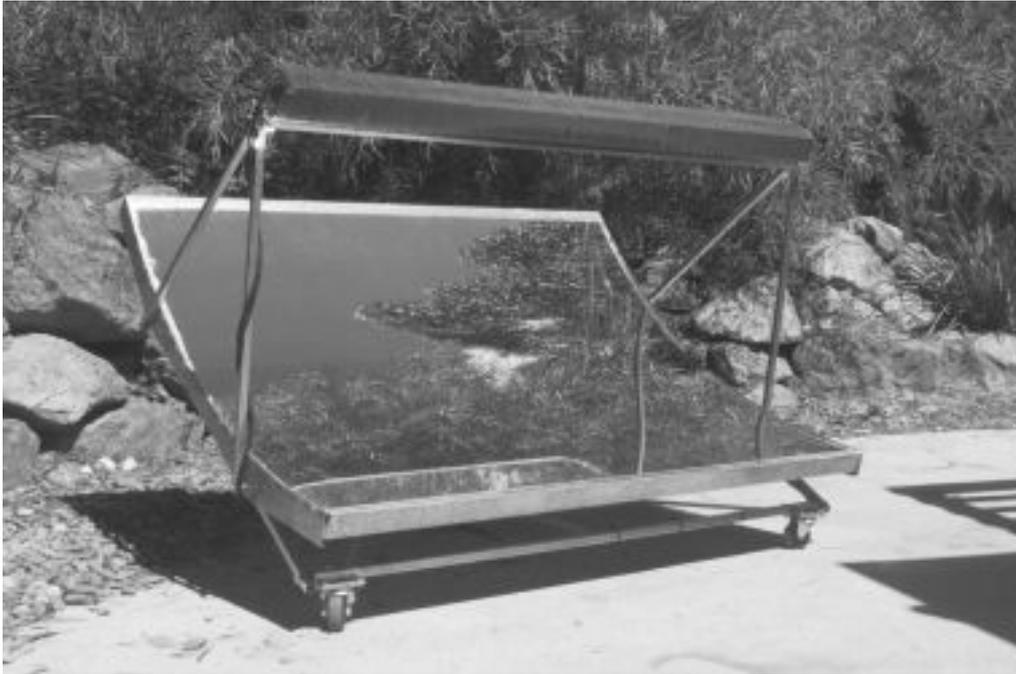
**Figure 5 Parabolic trough module**
