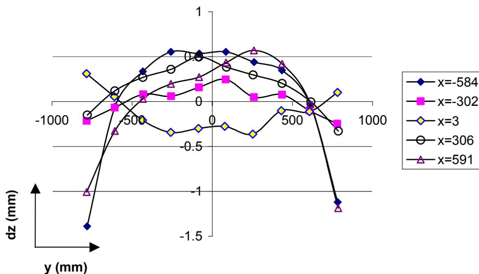
**Figure 6 Trough height deviation from ideal (trough z axis horizontal)**
