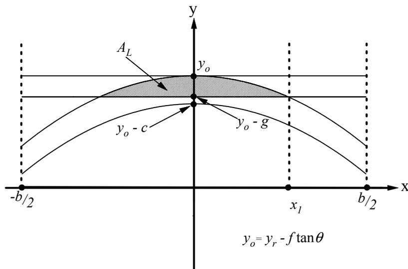
Figure 3 Intersection of flux source region and mirror gap
