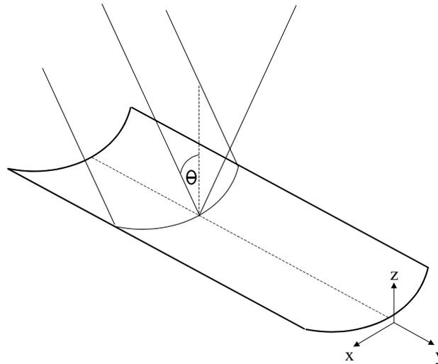
**Figure 1 Trough geometry with incident plane of rays**
