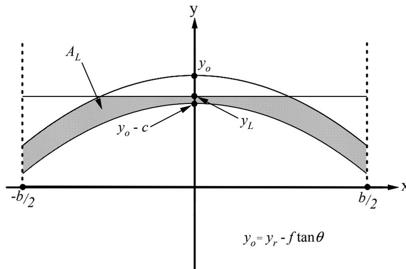
Figure 4 Flux loss due to mirror limit
