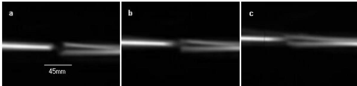
**Figure 8 Flux images for 45mm gap: 0° (a), 11° (b), and 23° (c) orientations.**
