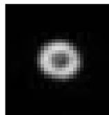
Fig. 3: Retro-reflective target with an annular reflectance pattern cause by surface dew.
