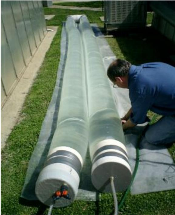
**Figure 5. 200 mm diameter tubes filled with water.**
