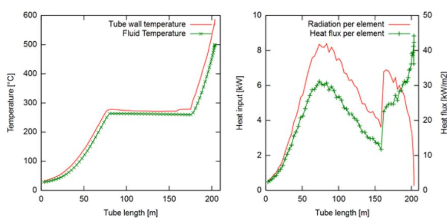
Figure 2: Temperature profile and heat flux distribution along tube length for a simplified receiver.
