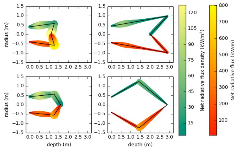
Figure 1. Examples of axisymmetric net radiative flux density (upper part of the profile) and net radiative flux (lower part of the profile) from ray-tracing simulations.
