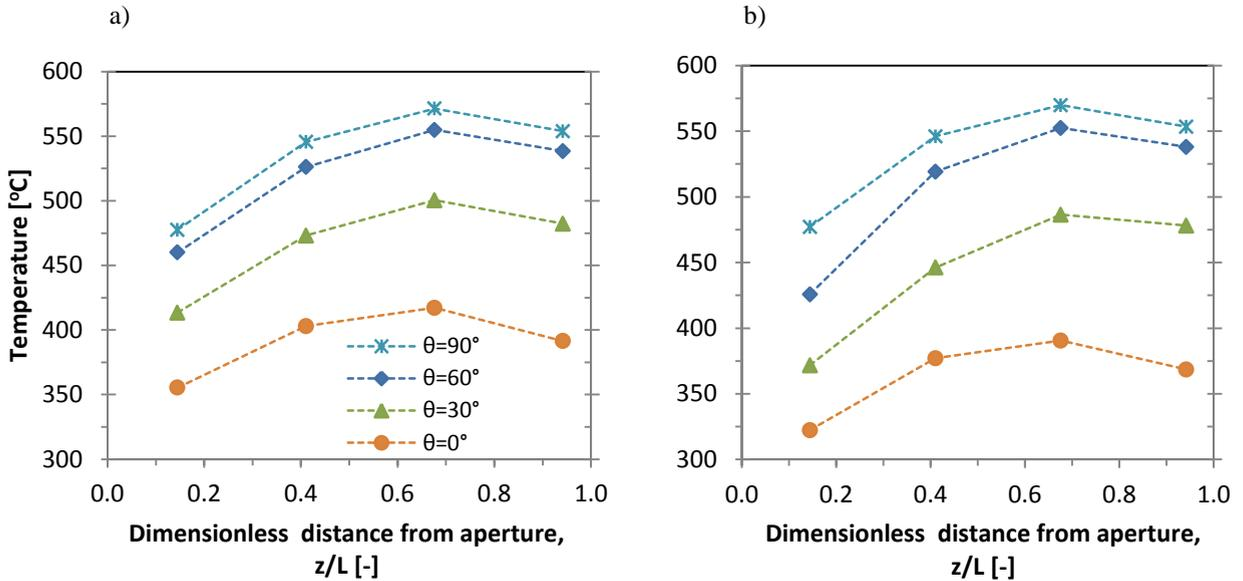
Fig. 4 Surface temperature distribution inside the cavity with AR=2,  $q=4260\text{W/m}^2$ : a) top surface. b) bottom surface. The legend in Fig. 4a can also be used for Fig. 4b
