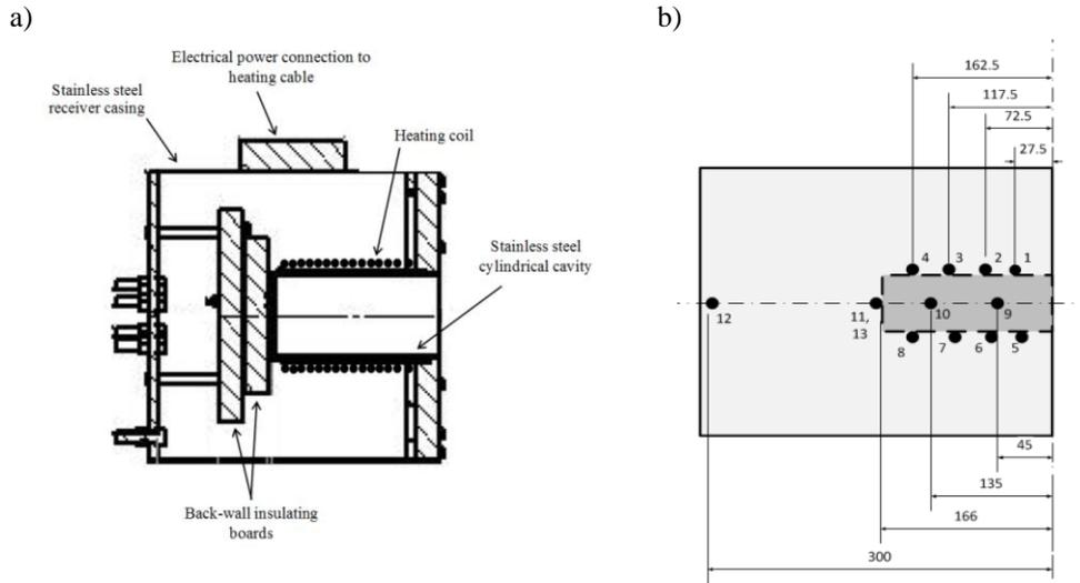
Fig. 3 Cross section sketch of lab-scale cavity receiver, showing a) different components of the receiver, b) thermocouple locations for cavity with  $AR=2$
